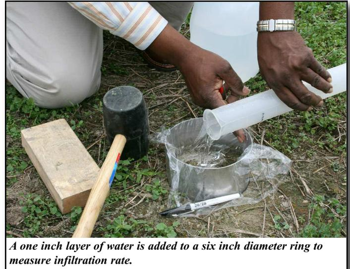
*A one inch layer of water is added to a six inch diameter ring to measure infiltration rate.*
